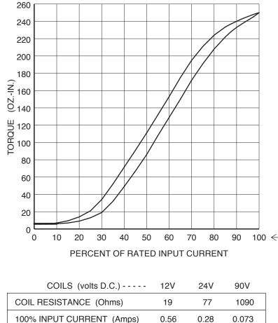
CHARACTERISTICS - With no electrical excitation, the shaft freely rotates. With electrical excitation, the shaft becomes coupled to the housing. Torque is proportional to input current (see torque graph), and independent of RPM. The brake will slip smoothly at the torque level set by the coil input current.
