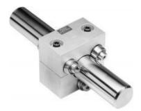
Zero- Max's Roh'Lix® linear actuators are threadless, mechanical, screw- type devices designed to convert rotary motion into precise linear motion and thrust using rolling element ball bearings. These adjustable automatic overload protectors will slip when overloaded, providing linear clutching without any additional clutch mechanisms.
